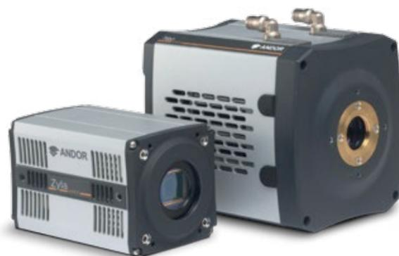
**Figure 2:** The Zyla is available in both 4.2 megapixel 'Zyla 4.2' and 5.5 megapixel 'Zyla 5.5' sensor formats. Both formats are available with either USB 3.0 or 10-tap interface. The 'Neo 5.5' features a 5.5 megapixel sensor, USB 3.0 interface and 4GB on-head memory buffer. Neo 5.5, Zyla 5.5 and Zyla 4.2 all produce data rates of up to ~850 MB/s at frame rates of 100 fps.
