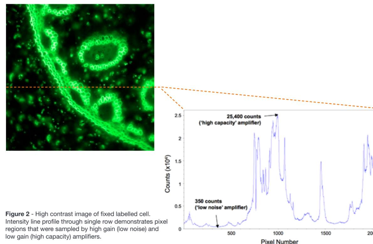
**Figure 2** - High contrast image of fixed labelled cell. Intensity line profile through single row demonstrates pixel regions that were sampled by high gain (low noise) and low gain (high capacity) amplifiers.
