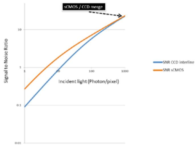
**Figure 5** - Theoretical Signal to Noise plot comparisons for sCMOS vs Interline CCD sensors. Photon flux (i.e. input light intensity) is given in terms of photons per 6.5 μm pixel of each sensor type.
