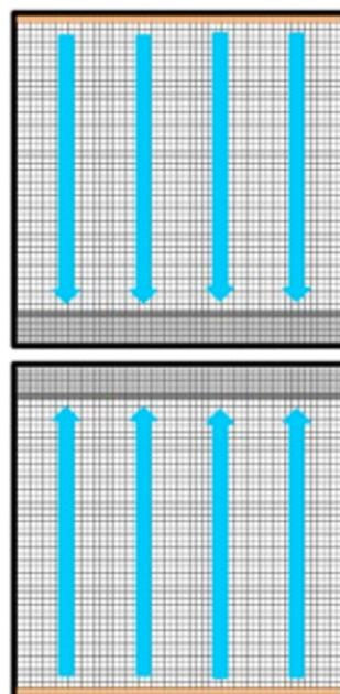
**Figure 2:** LightScan PLUS enables the rolling shutter to scan the sensor from top to bottom or vice versa in one continuous sweep. This is also known as "Single Port Readout"
