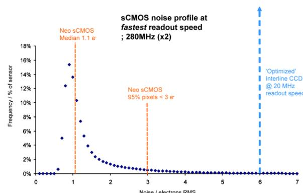
**Figure 1** - Representative histogram showing read noise distribution at fastest readout speed of 560 MHz. The median value of 1.1 e- means 50% pixels have less than 1 e- and 50% have greater than 1 e-. The line at 6 e- represents a typical read noise value from a well optimized Interline CCD – all pixels in a CCD share the same noise value.
