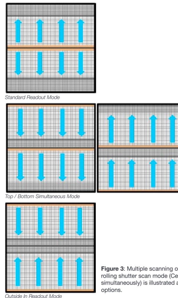
**Figure 3:** Multiple scanning options available. The standard rolling shutter scan mode (Center outwards in both directions simultaneously) is illustrated along with the three new scanning options.
