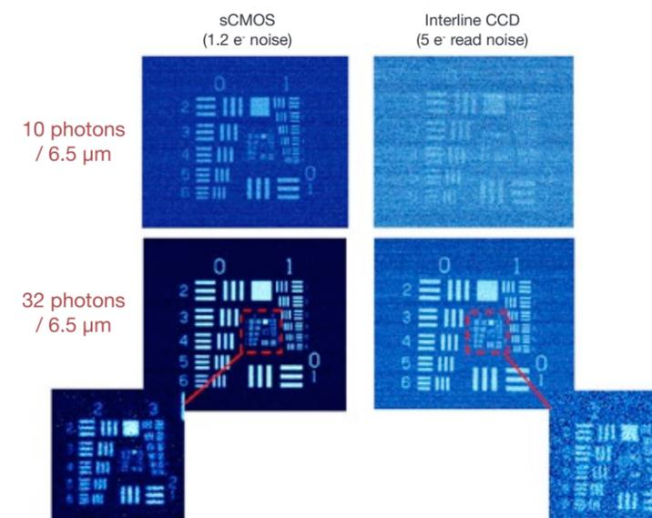
**Figure 1** - Comparative low light images of a USAF resolution chart, showing Andor sCMOS (1.3 electrons read noise @ 560 MHz) vs Interline CCD (5 electrons read noise @ 20 MHz), under the two lowest LED settings.
