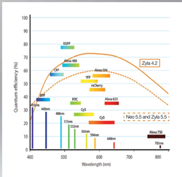
sCMOS Quantum Efficiency (QE) curves, incorporating laser excitation lines and emission ranges of common fluorophore labels.
