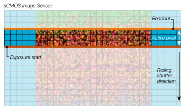
**Figure 1:** Rolling Shutter mode. The band of pixel rows in between is exposed to light simultaneously. This band moves from the top to the bottom of the sensor. Its width is defined by the single row exposure time, and can be adjusted from a minimum of one line up to the whole chip.
