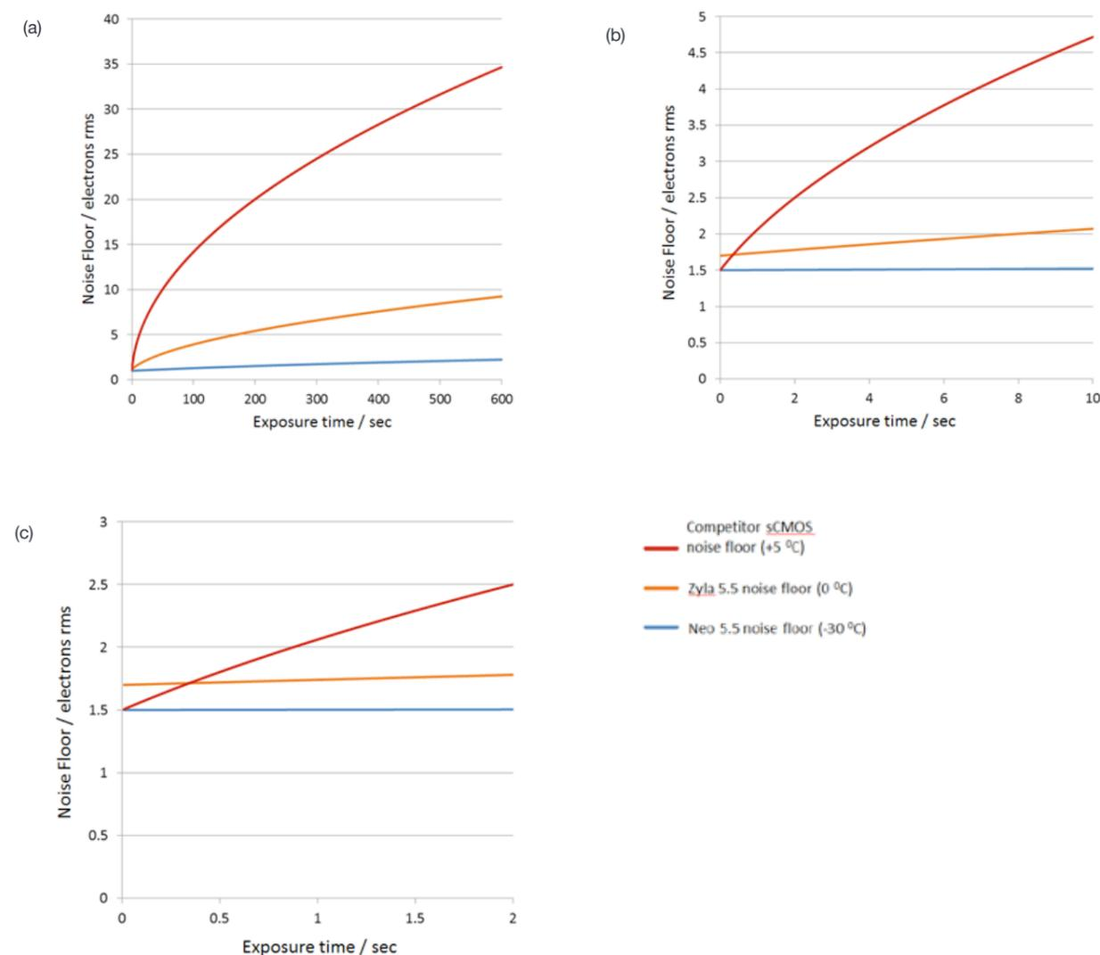
**Figure 1** - Plots of sCMOS noise floor (read noise and dark noise combined in quadrature) versus exposure time, for three different cameras all using the same 5.5 megapixel '5T' sensor type, cooled to their standard air cooled temperatures; a competitor's sCMOS camera cooled to +5°C, the Zyla 5.5 cooled to 0°C and the Neo 5.5. cooled to -30°C. Plots are displayed over three ranges of exposure time: 0 - 2 sec, 0 - 10 sec and 0 - 600 sec.
