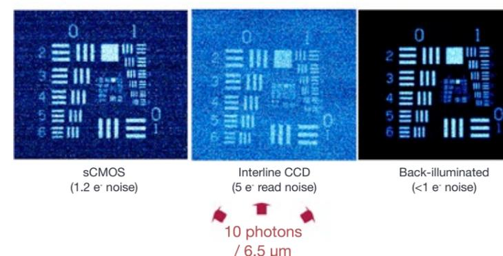
**Figure 2** - Comparative low light images taken with Andor sCMOS (1.3 electrons read noise @ 560 MHz) vs Interline CCD (5 electrons read noise @ 20 MHz) vs back-illuminated EMCCD (< 1 e<sup>-</sup> read noise), under extremely low light conditions (10 photons / 6.5  $\mu\text{m}$  setting). sCMOS and Interline CCD were 2 x 2 binned in order to have the same effective pixel pitch (and light collection area per pixel) as the 13  $\mu\text{m}$  pixel of the EMCCD sensor.
