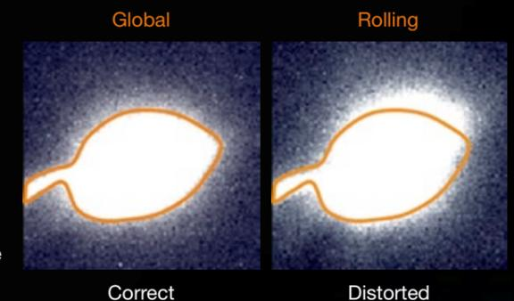
“ For our work on quantifying red blood cell velocity in the retinal capillaries we elected to operate in Global shutter mode, which produces minimally distorted images. When operating in Rolling shutter mode we observed significant image warping, even for moderate eye movements.
