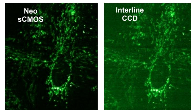
**Figure 3** - Comparative low light images taken with Andor sCMOS (1.3 electrons read noise @ 560 MHz) vs Interline CCD (5 electrons read noise @ 20 MHz) of fluorescently labelled fixed cell using a CSU-X spinning disk confocal microscope (x60 oil objective), each 100 ms exposure, same laser power, displayed with same relative intensity scaling. Note, the field of view is limited by the aperture size of the CSU-X, which is matched to the 1.4 megapixel Interline sensor.
