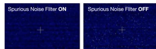
**Figure 2** - Demonstration of Spurious Noise Filter on a dark image, 20 ms exposure time, 200 MHz (x2) readout speed (~1.2 e- read noise).
