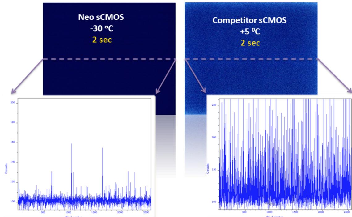
**Figure 2** - Thermal noise can sacrifice the sCMOS low detection limit. Low light images recorded with a Neo sCMOS at -30°C versus a competing sCMOS using the same sensor, operated at +5°C. Shown with same relative intensity scaling; 2 sec exposure time; 560MHz readout speed. Comparative line intensity profiles from a single row is also shown for each case.
