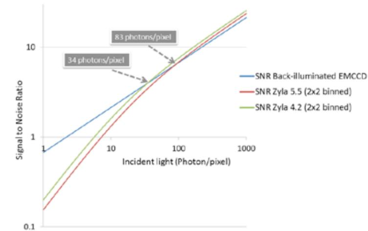
**Figure 6** - Plot of Signal to Noise Ratio versus Incident Photon Intensity, comparing back-illuminated EMCCD iXon 888 (13 μm pixel size) to 2x2 binned Zyla sCMOS cameras (13 μm pixel size after binning). An average QE value for each sensor between 500-750 nm was used.
