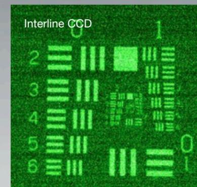
Comparative low light images taken with Neo sCMOS (1.3 electrons read noise @ 560 MHz) vs. Interline CCD (5 electrons read noise @ 20 MHz), displayed with same relative intensity scaling.
