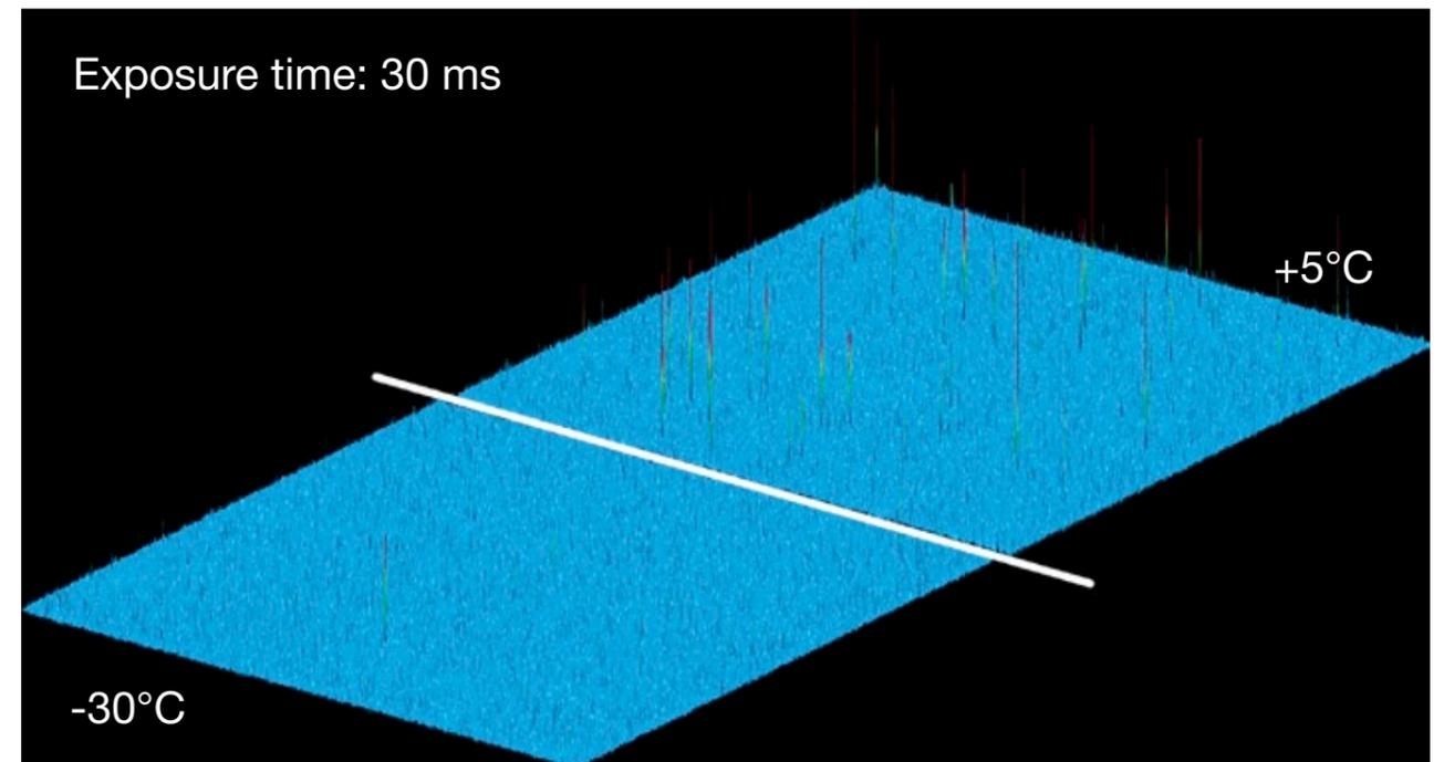
**Figure 3 (b)** – Blemishes at -30°C vs +5°C for 30 ms exposure.
