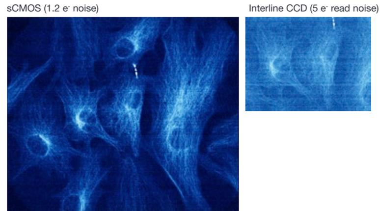
**Figure 4** - Comparative low light fluorescence microscopy images taken with Andor sCMOS (1.3 e<sup>-</sup> @ 560 MHz) vs Interline CCD (5 e<sup>-</sup> @ 20 MHz) under low light conditions, typical of those employed in dynamic live cell imaging. ND filters on a widefield fluorescence microscope were used to reduce light levels relative to the read noise floor.
