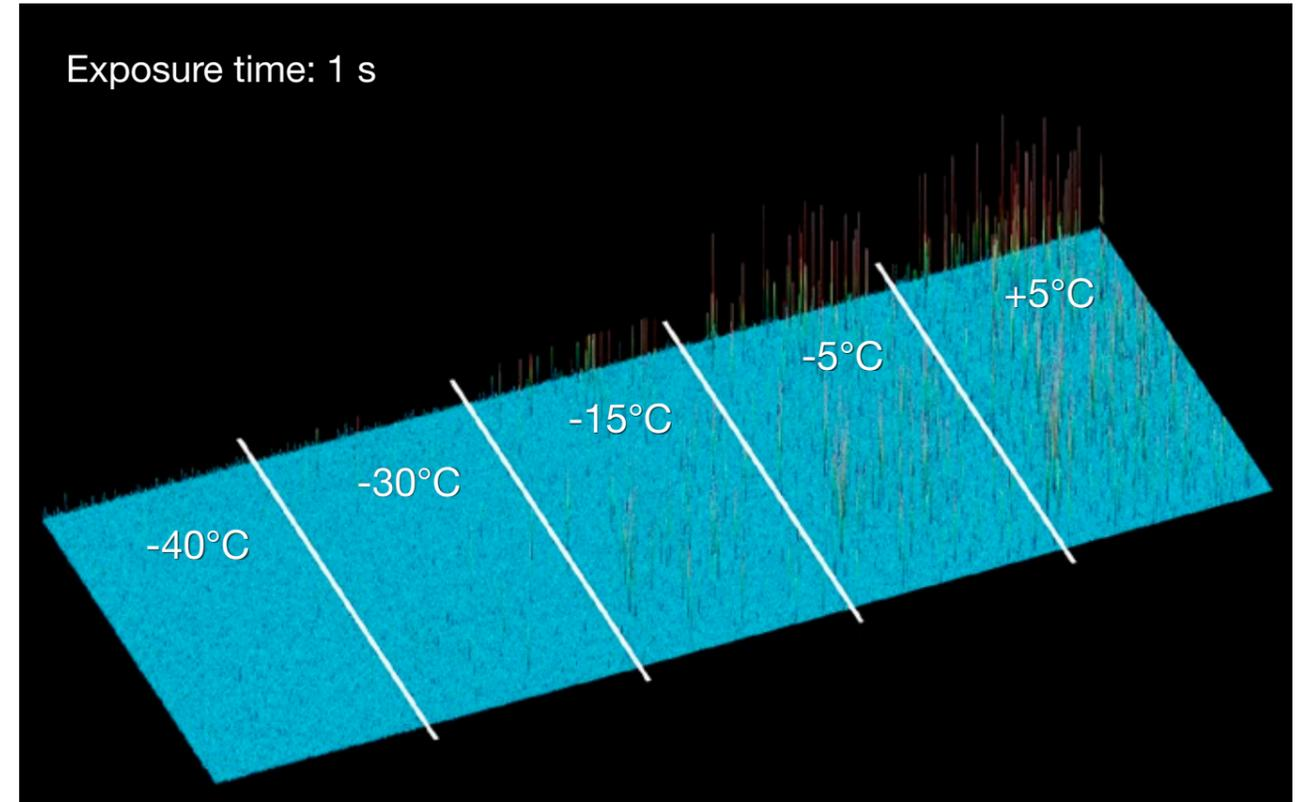
**Figure 3 (a)** – Blemishes at different temperatures for 1 sec exposure.
