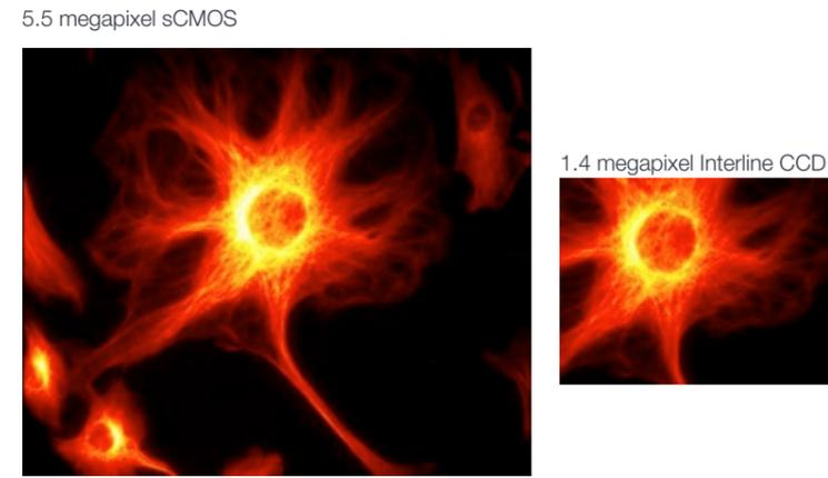
**Figure 7** - Field of view comparison of two technologies; x60 magnification, 1.25 NA, 5.5 megapixel Andor sCMOS vs 1.4 megapixel Interline CCD (each have ~6.5 μm pixel pitch). sCMOS is capable of offering this larger field of view @ 100 frame/s with 1.3 e<sup>-</sup> read noise.
