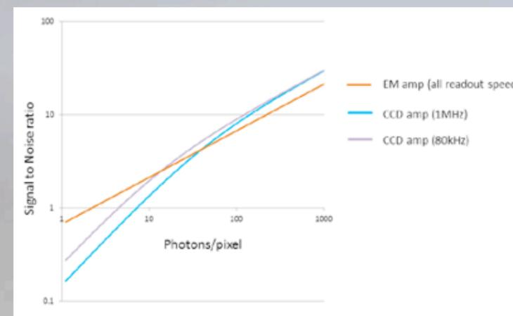
Signal to Noise plots, comparing EMCCD mode at any readout speed vs CCD mode at 1 MHz and 80 kHz readout speeds (the latter exclusive to iXon Ultra 897). Higher signal to noise can be secured with the 80 kHz CCD amplifier for light levels greater than 12 photons/pixel, but note that this corresponds to a max frame rate of 0.3 fps.
