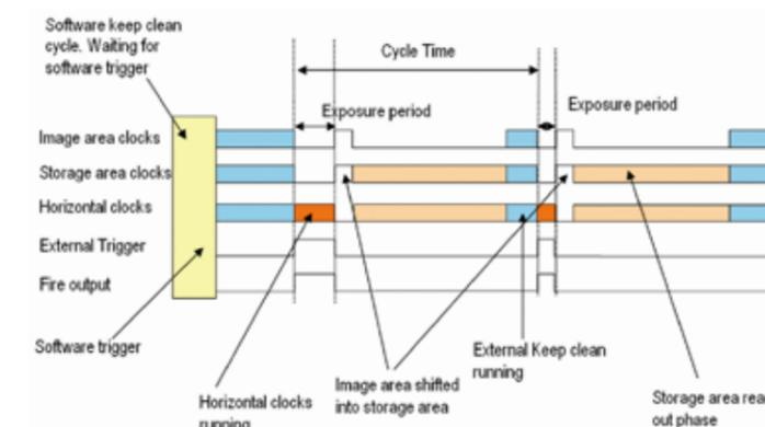
Figure 3: External Exposure in non-Frame Transfer mode
