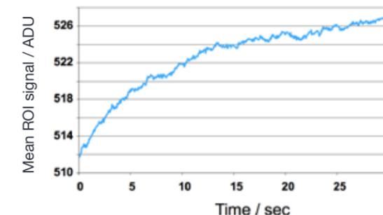
Figure 1 - iXon Baseline Clamp (bias stability) in operation. A standard feature in iXons since 2002.
