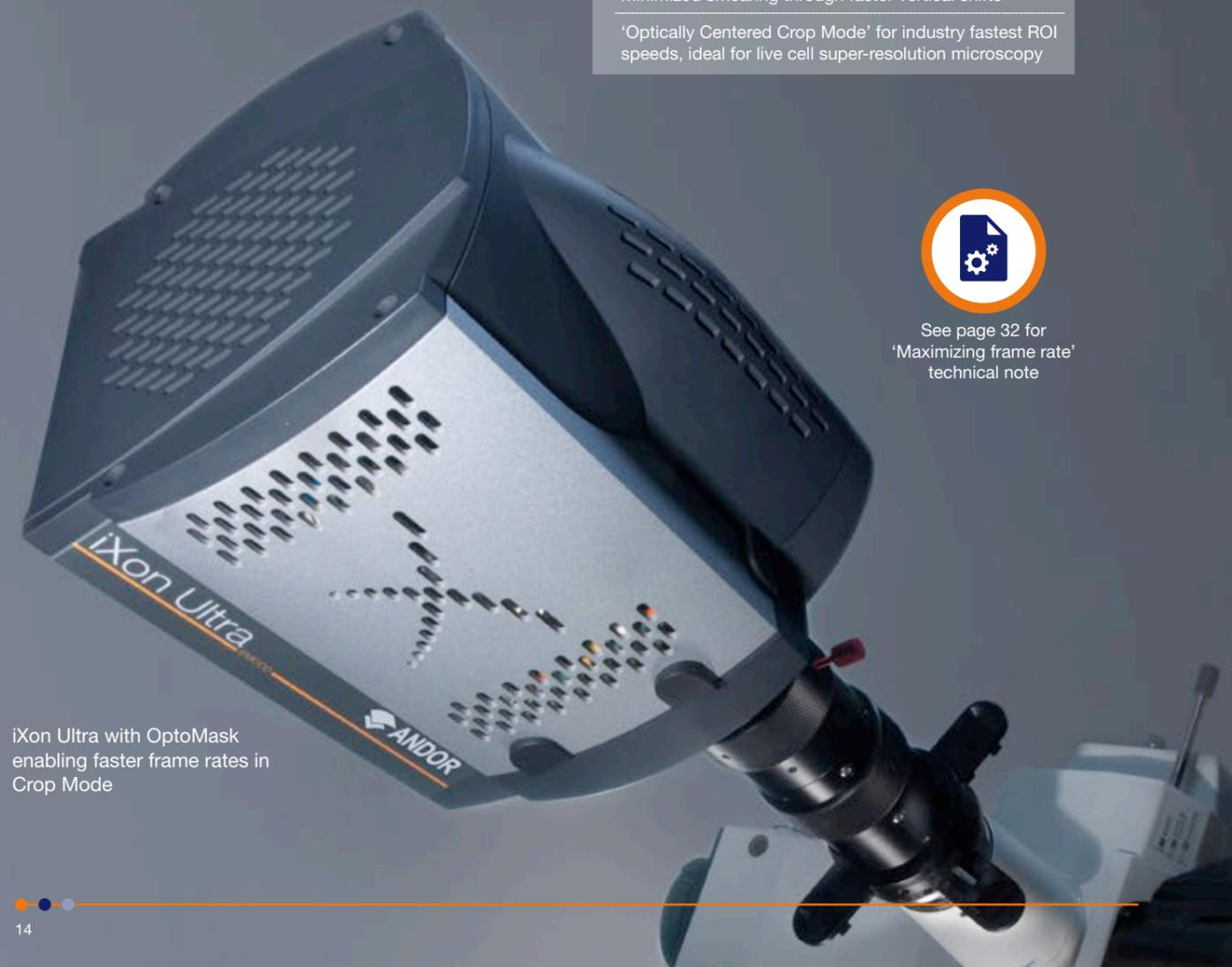
iXon Ultra with OptoMask enabling faster frame rates in Crop Mode
