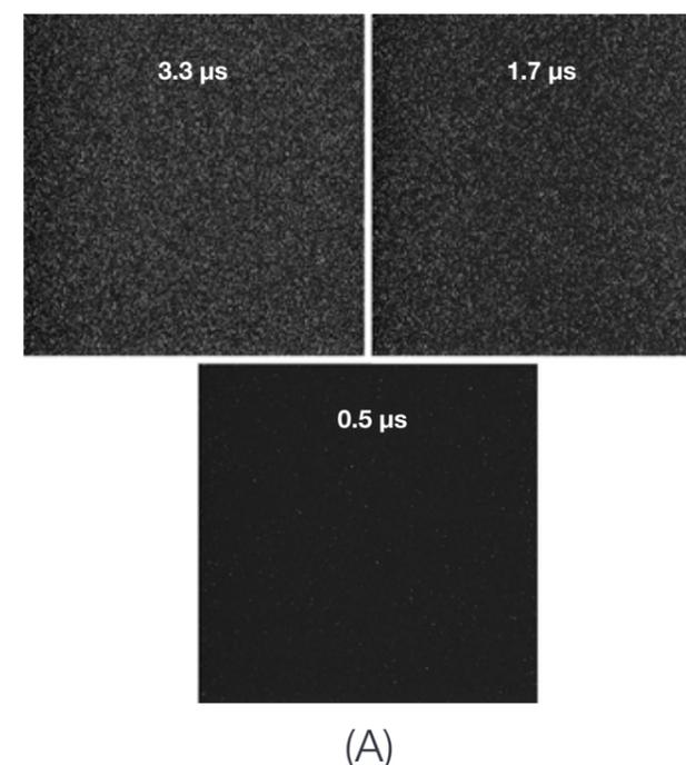
You can see that the vertical clock speeds have a significant impact on further reducing CIC, with the speed of 0.5 μs/shift offering the lowest CIC and therefore highest EMCCD sensitivity. This iXon3 clock speed performance is faster than other EMCCDs in the industry.
