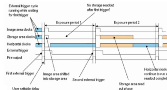
Figure 1: External Trigger in Frame Transfer mode
