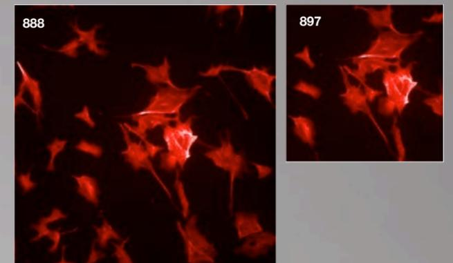
Field of View Comparison between iXon Ultra models. The 888 model has a x2.6 greater sensitive area than the 897 model.
