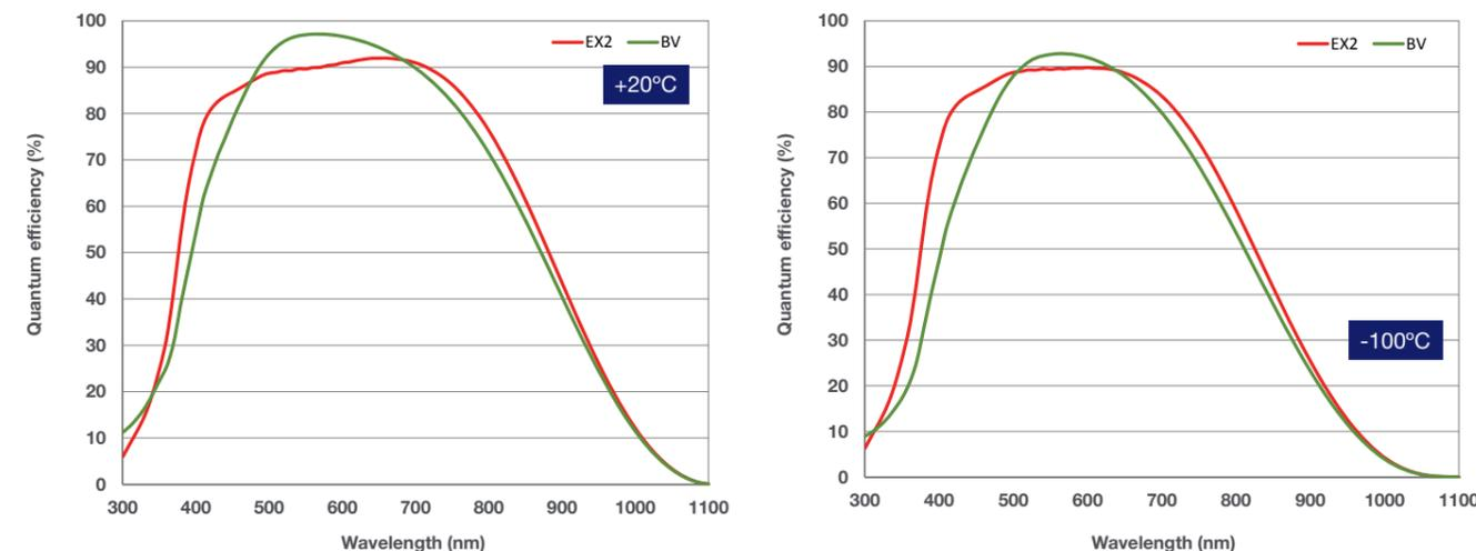
**Figure 1:** Back-illuminated EMCCD sensor QE curves, comparing standard 'BV' mid-band AR coating versus new EX2 dual AR coating. Reference data available at +20°C and -100°C sensor cooling temperatures.
