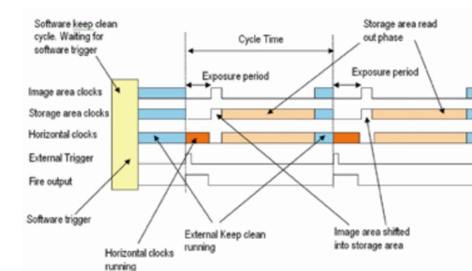
Figure 2: External Trigger in non-Frame Transfer mode
