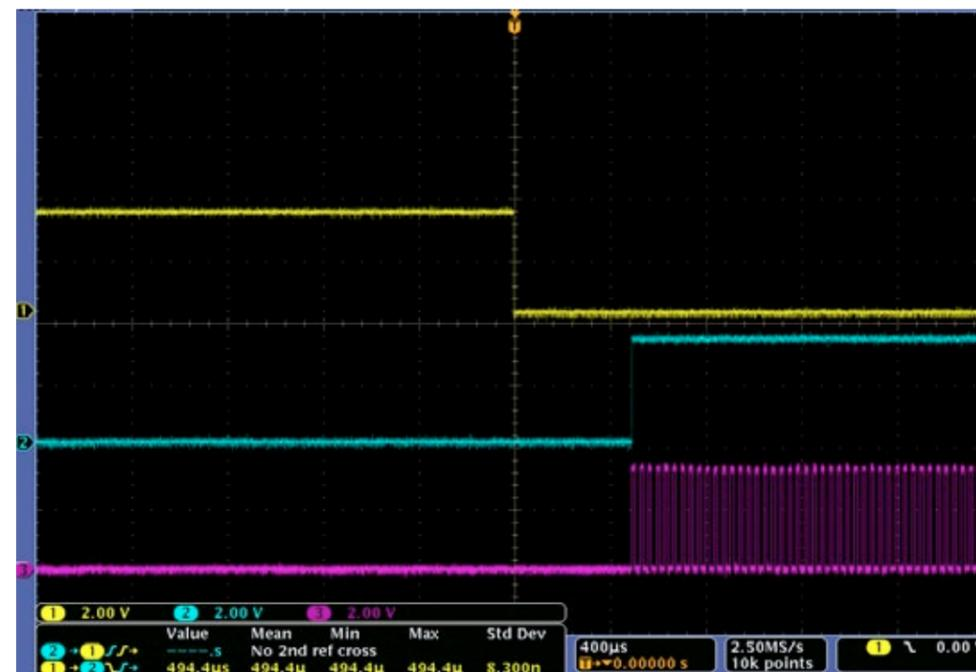
Figure 1: Latency – Vertical shift rate = 0.5 $\mu$ s, Time from falling edge of FIRE to rising edge of Camera Link FRAME = 494.4 $\mu$ s (268 $\mu$ s of this time is the time required to shift the image into the mask area of the sensor). Ch1: Camera FIRE (Yellow); Ch2: CL FVAL (Blue); Ch3: CL LVAL(Pink)
