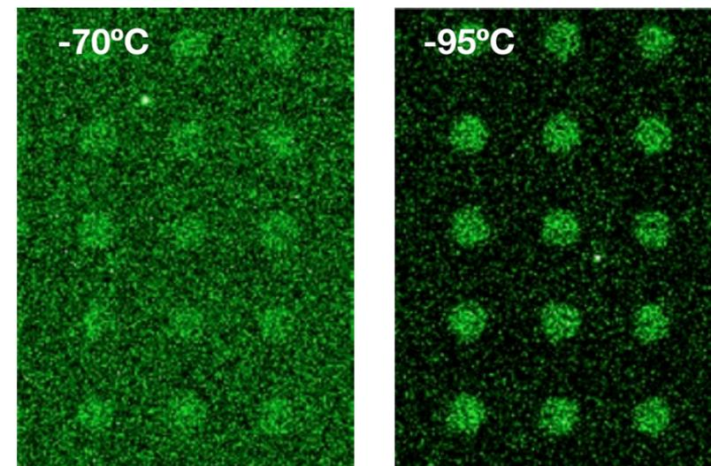
**Figure 2:** Images of extremely weak LED signal (signal intensity typical of weak luminescence experiments) acquired with iXon 888 at cooling temperatures -70°C and -95°C (water cooling to achieve latter), 120 sec exposure times, sub-region show. The need to push to such deep cooling temperatures can be readily observed under such extreme low light conditions.
