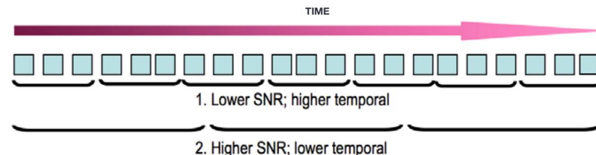
**Figure 2 – Schematic illustration of how photon counting can be applied to a kinetic series as a post processing step, affording increased flexibility in 'trial and error' trading SNR vs temporal resolution.**
