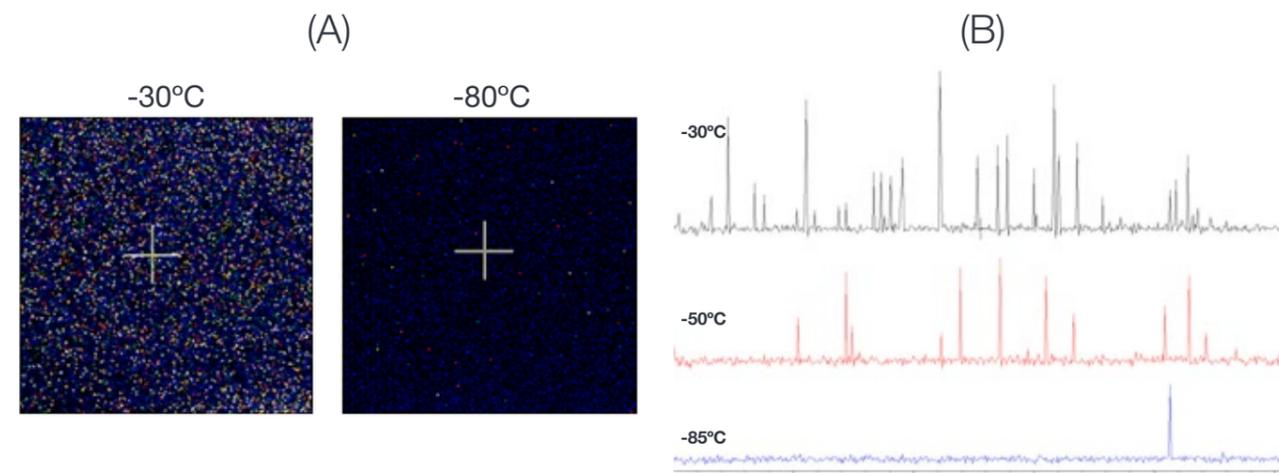
**Figure 1:** (A) shows dark images taken at x1000 gain at different cooling temperatures, 29 ms exposure time. Vertical shift speed was 0.5  $\mu$ s/row to ensure minimal CIC. (B) shows typical line intensity profiles across a row of 512 pixels, taken from such dark images at three different cooling temperatures. The cleanest noise floor is clearly seen under conditions of deep cooling, even for such short exposure times.
