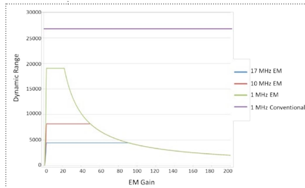
**Figure 1** – Dynamic Range vs EMCCD gain, for iXon Ultra 897. Shown for EM amplifier @ 17, 10 and 1 MHz readout speed and for Conventional amplifier at 1 MHz readout speed. Well capacities used in DR calculation are characteristic of the CCD97 512 x 512 back-illuminated L3 sensor from e2v. Dynamic range only exceeds 14-bits max @ 1 MHz, through either amplifier.
