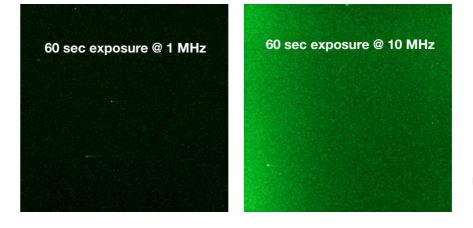
**Figure 3:** Dark noise background at 1 MHz and 10 MHz readout speeds; 60 sec exposure and -70°C cooling.
