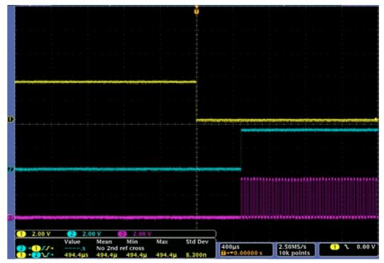
Figure 1: Latency – Vertical shift rate = 0.5 µs, Time from falling edge of FIRE to rising edge of Camera Link FRAME = 494.4 µs (268µs of this time is the time required to shift the image into the mask area of the sensor). Ch1: Camera FIRE (Yellow); Ch2: CL FVAL (Blue); Ch3: CL LVAL(Pink)
