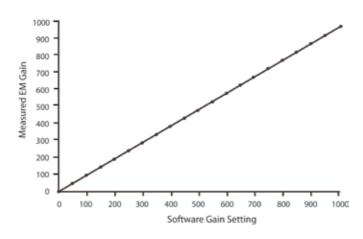
Figure 1 – RealGain™ calibration in the iXon – the same linear relationship holds across all cooling temperatures.
