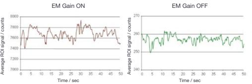
Figure 3 - Instability of the light source on a standard research grade epifluorescence microscope.
