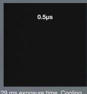
DARK IMAGES taken with the iXon3 897 at x1000 gain at different vertical shift speeds, 29 ms exposure time. Cooling temperature was -85°C to ensure minimal dark current contribution.
