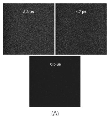
You can see that the vertical clock speeds have a significant impact on further reducing CIC, with the speed of 0.5 µs/shift offering the lowest CIC and therefore highest EMCCD sensitivity. This iXon3 clock speed performance is faster than other EMCCDs in the industry.
