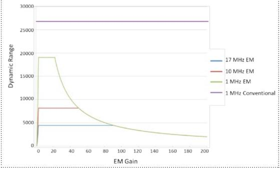
Figure 1 – Dynamic Range vs EMCCD gain, for iXon Ultra 897. Shown for EM amplifier @ 17, 10 and 1 MHz readout speed and for Conventional amplifier at 1 MHz readout speed.
