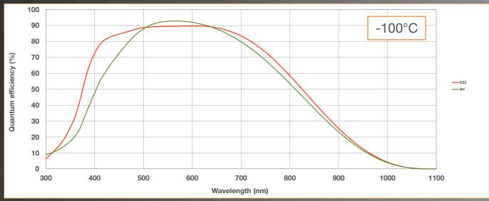
Back-illuminated EMCCD sensor QE curves, comparing standard 'BV' mid-band AR coating versus new EX2 dual AR coating. Reference data available at +20°C and -100°C sensor cooling temperatures.
