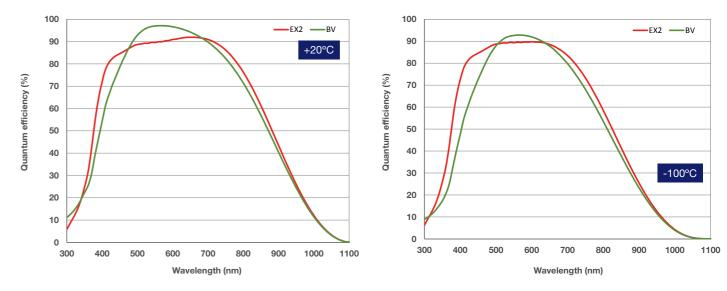
Figure 1: Back-illuminated EMCCD sensor QE curves, comparing standard 'BV' mid-band AR coating versus new EX2 dual AR coating. Reference data available at +20°C and -100°C sensor cooling temperatures.
