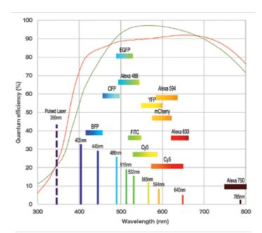
QE curves of iXon models vs emission of common fluorophores
