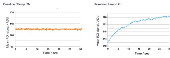
Figure 1 - iXon Baseline Clamp (bias stability) in operation. A standard feature in iXons since 2002.
