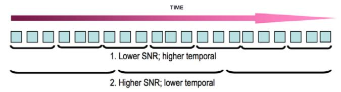
Figure 2 – Schematic illustration of how photon counting can be applied to a kinetic series as a post processing step, affording increased flexibility in 'trial and error' trading SNR vs temporal resolution.
