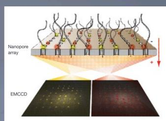
Schematic diagram of the single molecule Optipore sequencing method, with an illustration of the 'enzyme-free' nanopore array through which DNA strands are electrophoretically drawn. iXon3 860 cameras were used to capture two color sequencing data at 1000 fps.
