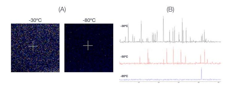
**Figure 1:** (A) shows dark images taken at x1000 gain at different cooling temperatures, 29 ms exposure time. Vertical shift speed was 0.5 µs/row to ensure minimal CIC. (B) shows typical line intensity profiles across a row of 512 pixels, taken from such dark images at three different cooling temperatures. The cleanest noise floor is clearly seen under conditions of deep cooling, even for such short exposure times.
