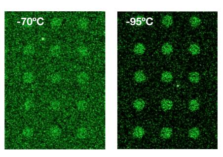
Figure 2: Images of extremely weak LED signal (signal intensity typical of weak luminescence experiments) acquired with iXon 888 at cooling temperatures -70°C and -95°C (water cooling to achieve latter), 120 sec exposure times, subregion show. The need to push to such deep cooling temperatures can be readily observed under such extreme low light conditions.
