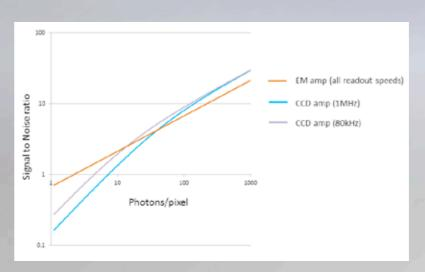
Signal to Noise plots, comparing EMCCD mode at any readout speed vs CCD mode at 1 MHz and 80 kHz readout speeds (the latter exclusive to iXon Ultra 897). Higher signal to noise can be secured with the 80 kHz CCD amplifier for light levels greater than 12 photons/pixel, but note that this corresponds to a max frame rate of 0.3 fps.
